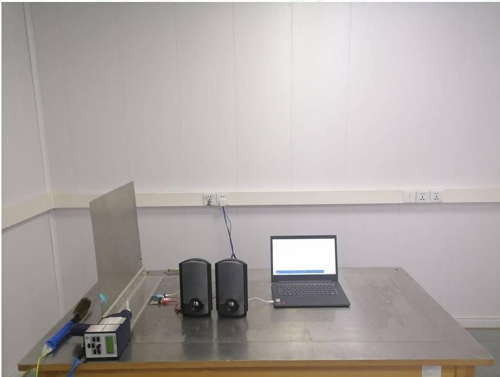
Test Setup Photo of Electrostatic Discharge Test
